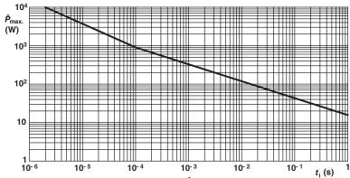
Pulse on a regular basis; maximum permissible peak pulse power  $\hat{P}_{max}$  as a function of pulse duration (*t*<sub>i</sub>) for single pulse condition
