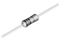
A metal glazed film is deposited on a high grade ceramic body. After that caps are applied to the rods and tinned electrolytic copper wires are welded to these end caps.
